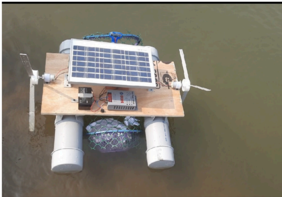
FIG. 3. EXPERIMENTAL SETUP OF SOLAR BASED WI-FI RIVER CLEANING ROBOT
